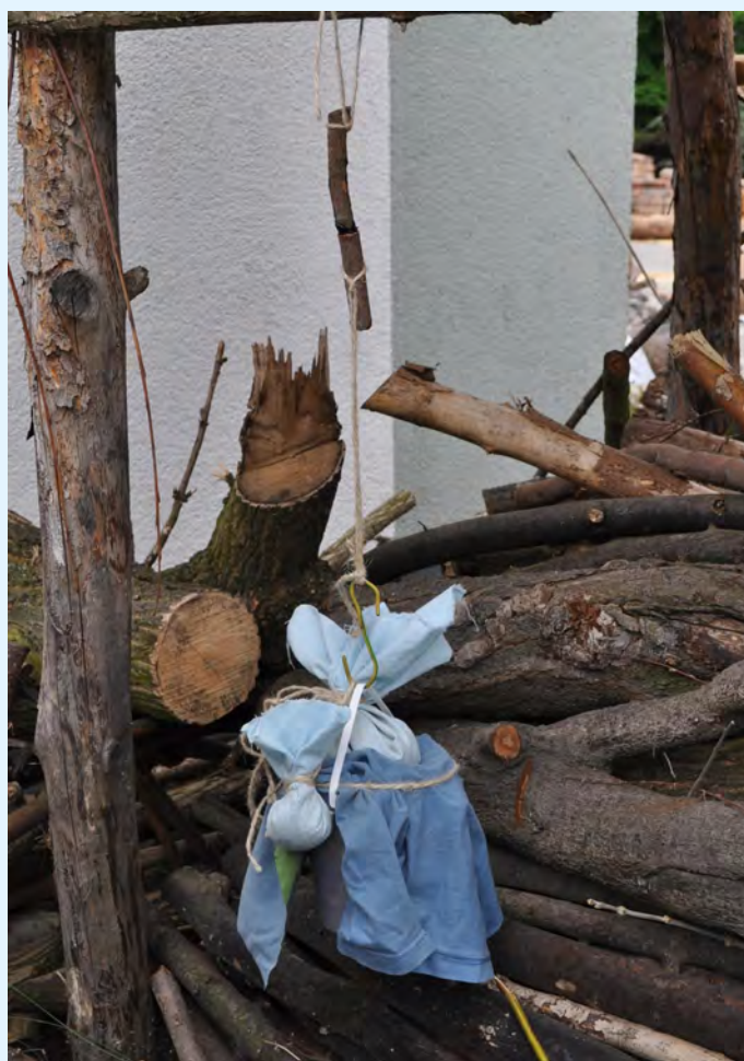
Fig.3 Example of one of conducted strength tests consisted in applying under bonded elements a load of increasingly greater weight and examining the load that joint could withstand.
