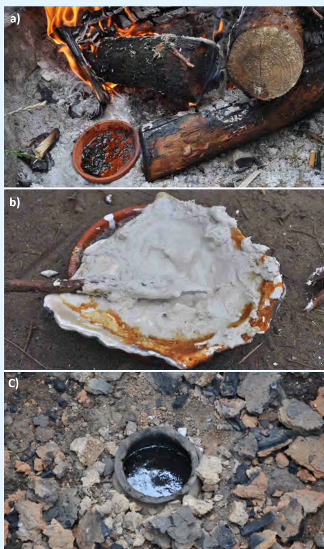
Fig.1 Examples of used during experiments adhesives: a) pine resin mixed with charcoal; b) adhesive made from milk and vinegar with the addition of calcium; c) tar obtained by means of the two-vessel method.
