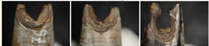
TYPE III - PERFORATION MADE BY SCRAPING AND DRILLING
